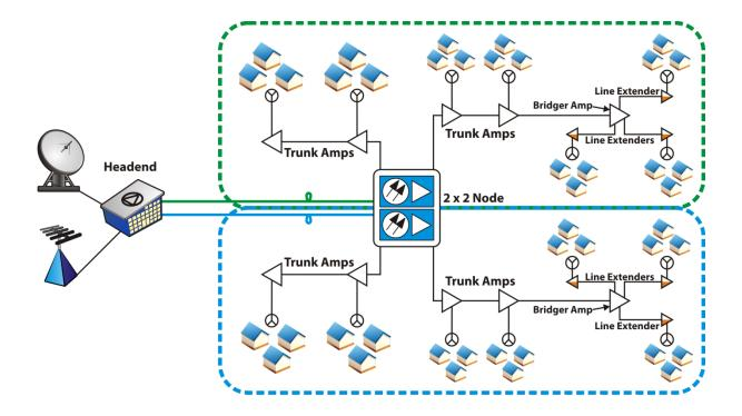
Bridger Upgrade Using OM3101 Reduces Amplifier Cascades, Drives Fiber Deeper
