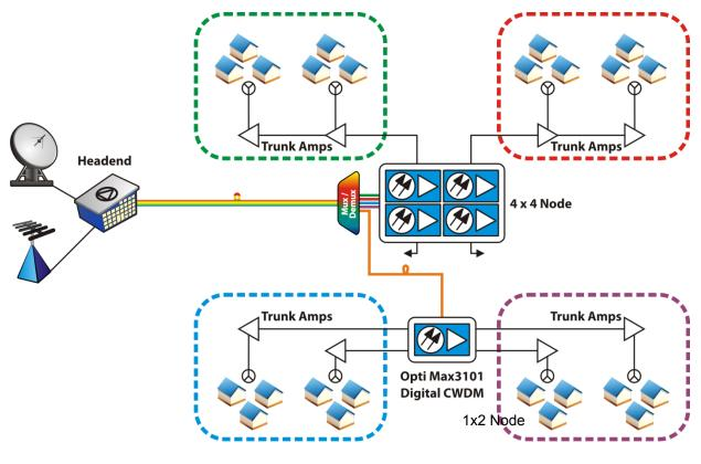
Fnd with: Full 2 x 2 Downstream and Unstream Segmentation using OM3100 as a replacement
