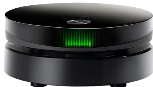
VIP4205 with the ARRIS DVR-One USB hard drive fitted underneath for DVR services.
